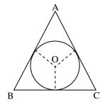
The radius of this circle is always denoted by r and is equal to the length of the perpendicular from its centre to any one of the sides of triangle.
